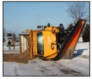
(This photo illustrates what can happen when the plow digs into a soft shoulder. The plow trips the truck, causing it to careen out of control. **NOTE:** This was an actual plowing accident. No trick or staged photography was used for this article.)
