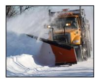
(The photo above illustrates the front plow elevated a few inches to allow for safe and effective plowing. **NOTE:** The plow shoe is being used and adjusted properly.)
