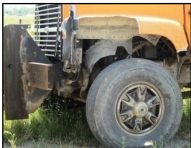
(Truck Fender Damage from a Tire Blow Out)
