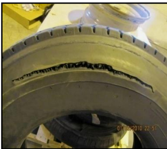
(Vehicle Tire Zipper Rupture)
