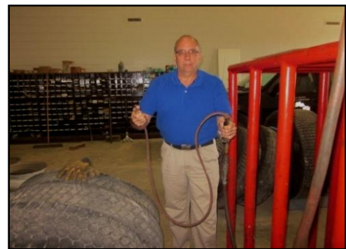
(Tire Inflation Gun with a Six Foot Air Line)
