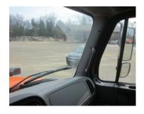
5. Backing Maneuvers - Objects can be hidden behind a snowplow truck. Remember that the dead space can range from a distance of 80-90 feet behind your truck. This distance can be identified with a simple dead space demonstration. We encourage drivers to avoid having to back up whenever possible, keeping in mind that if the motorist cannot see your mirrors, you are likely not seeing the motorist!
