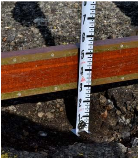
Using a tape measure and level in close-ups can help provide objective evidence.
