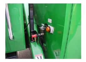
Recently, a MCRCSIP member reported that a truck electrical fire was subdued when the driver noticed smoke coming from the underside of the vehicle. The quick-thinking driver shut off the vehicle battery disconnect switch, helping to bring the fire under control. We believe his quick actions saved the truck and (most likely) the garage from extensive fire damage! It goes without saying that a special "Thank You" goes out to the truck driver, **Bill**
